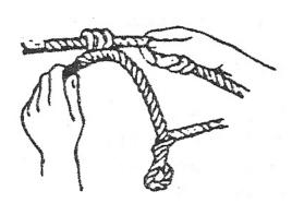
**F.** Pass the long end of the rope through the loop splice and your halter is complete.
