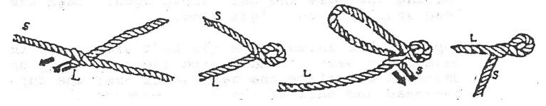
**D.** Take the short end of the rope in your left hand and with the right hand 2-3 inches from the left, untwist and push together until the strands form separate loops.
