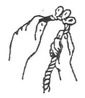
**E.** Work these loops into a straight line and pass the long end of the rope through these loops in the direction shown to form the adjustable head stall.
